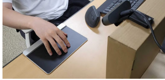
Figure 14: Collecting fingertip pressure data from a Sensel pad and hand data from an RGB camera to quantitatively evaluate PressureVision++ and our model.
